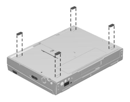
Figure 5-16. Installing the Computer Feet
